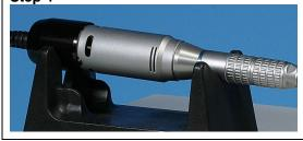
Push the straight nose cone onto the rod of the micro-motor until it snaps into place.
